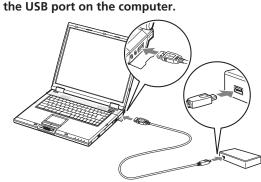
The computer recognizes the reader/writer as a removable disk, and the reader/writer is ready for use.
